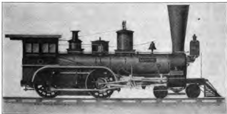
Fig. 116. Trenton Locomotive for Belvidere & Delaware Railroad, 1855, with Allan Link Motion
