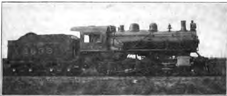
Modern 2-8-0 Freight Engine, on Canadian Pacific Railway. Cylinders, 21x28 Inches Drivers, 57 Inches; Weight of Engine, 186,200 Pounds; Steam Superheated
