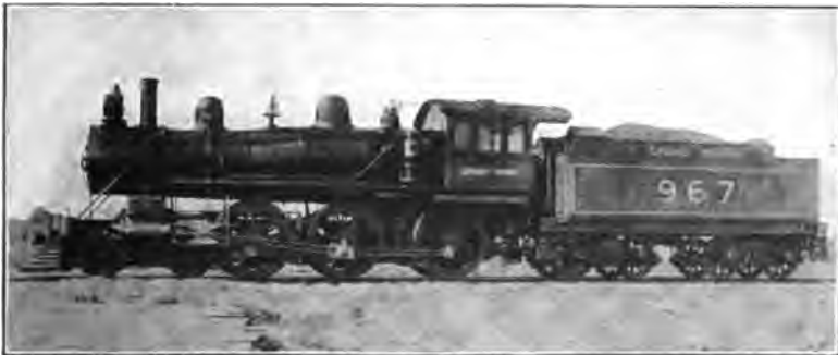
Modern Ten-Wheel Passenger Engine, Built by Grand Trunk Railway, Montreal Shops. Cylinders, 20x26 Inches; Drivers, 73 Inches; Weight of Engine, 182,000 Pounds
