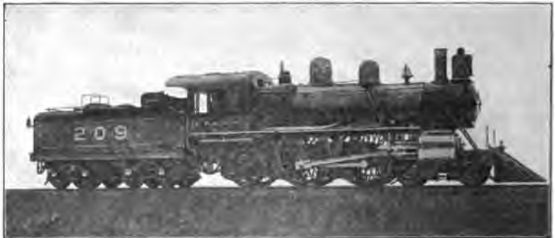
Modern Vaucain 4-Cylinder Compound Passenger 4-4-2 Engine, Built at Canadian Pacific Shops, Montreal, in 1898. Cylinders, 13\frac{1}{2} and 23 x 26 Inches; Drivers 84 Inches; Weight of Engine, 170,250 Pounds
