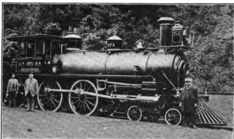
Fig. 140 "Audenried," with Clark's Independent Cut Off
