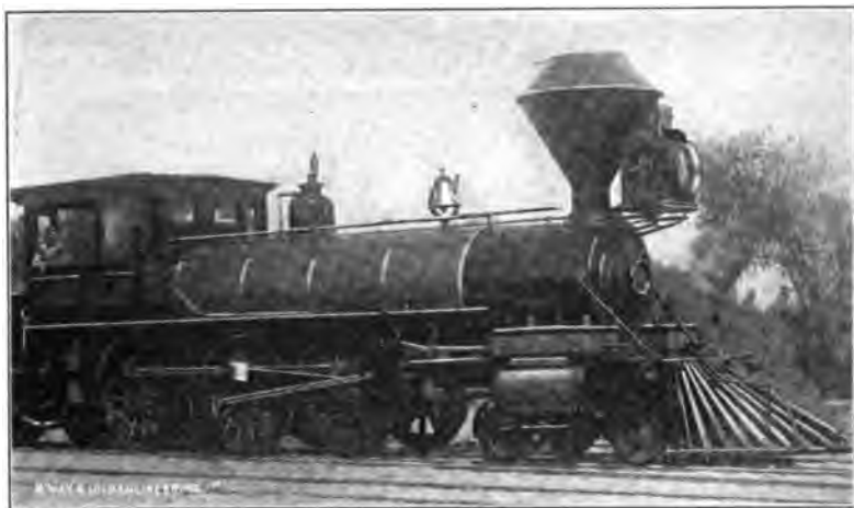
Southern Pacific Engine, with Stevens Valve Motion, 1885
