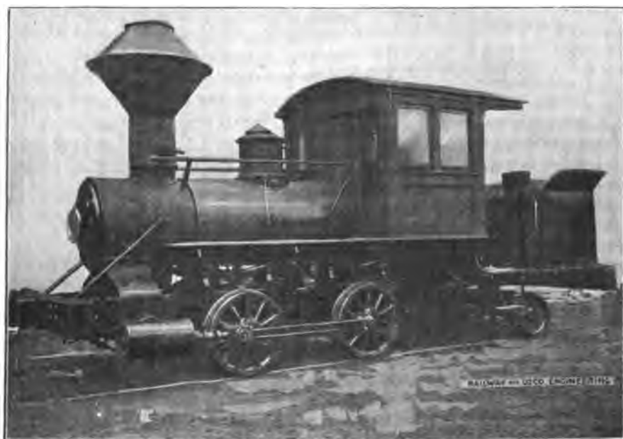
Fig. 268. Engine with Oscillating Cylinder and No Valve Gear
