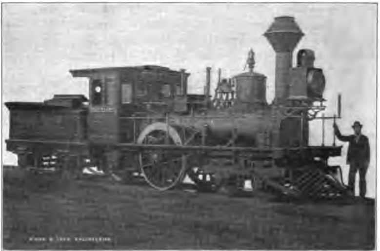
Fig. 86. Lowell Engine, Built About 1837, Rebuilt 1846, Belonged to Stonington Railroad. James M. Anderson, Master Mechanic of Road, in Front
