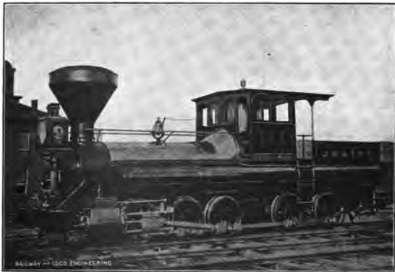
Special Grade-Climbing Locomotive, Designed and Built by Reuben Wells
