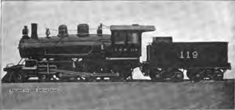
Modern 4-6-0 Passenger Engine, for the Intercolonial Railway, Built in 1899, at Canadian Locomotive Works, Kingston, Ont Cylinders, 20 x 26 Inches Drivers, 72 Inches ; Weight of Engine, 145,000 Pounds
